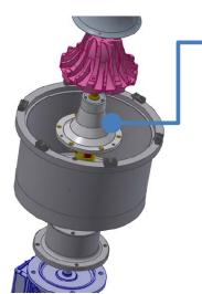
Direct drive with independent double-bearing system
